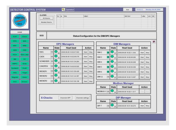
The DCS panel, accessible by clicking the "DCS" button on the left, shows the state of the servers used for monitoring/control of equipments (GREEN: running; RED: stopped). "Start/Stop" buttons can be used by the shift crew to restart managers that stopped for some reason. One should wait a few minutes until the manager is restarted and the bullet turns GREEN. If it does not work, call a DCS expert (#164872).
